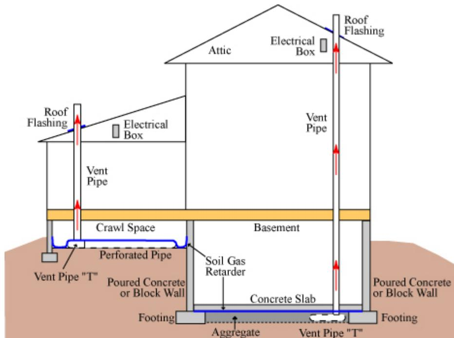
Additionally, all potential soil gas entry points are sealed with caulking or expanding foam and the basement walls are waterproofed. Common entry points that require sealing include floor/wall joints, gaps around pipes, plumbing, sump pits and the tops of block walls.
